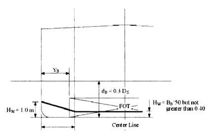
$B_B/5$  or 11.5 metres, whichever is less (measured inboard from the ship's side at right angles to the centerline at the level  $d_B$ )
